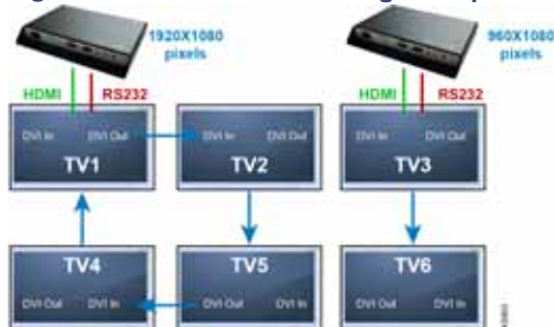
Figure 8 Video Wall Cabling Example Using TV Tile Matrix Functionality
