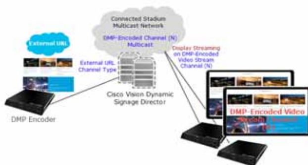
Figure 7 External URL Example with Display Streaming to a DMP-Encoded Multicast Channel
