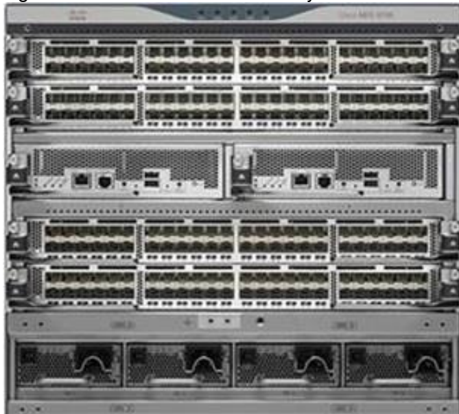
Figure 9 Cisco MDS 9706 Multilayer Director Front Side View
