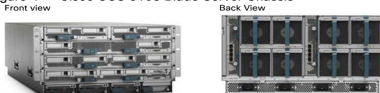
Figure 4 Cisco UCS 5108 Blade Server Chassis
