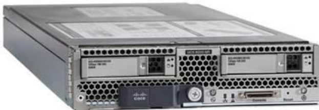
Figure 5 Cisco UCS B200 M5 Blade Server
