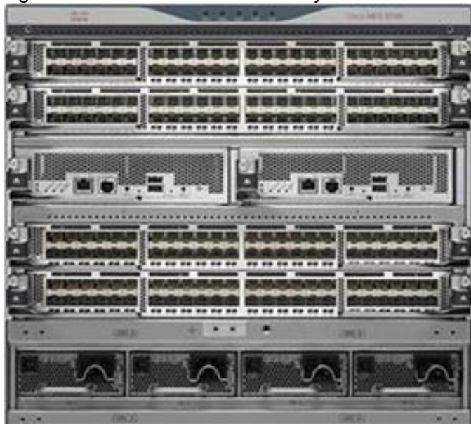
Figure 31 Cisco MDS 9706 Multilayer Director Front Side View
