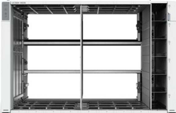
Figure 3. Cisco UCS X9508 Chassis - Midplane Free Design
