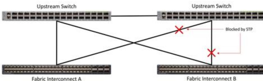
Figure 27. Connectivity with Multiple Uplink Switches
