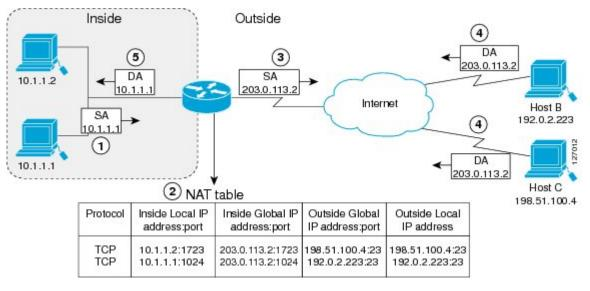
The device performs the following process in the overloading of inside global addresses, as shown in the preceding figure. Both Host B and Host C believe that they are communicating with a single host at address 203.0.113.2. Whereas, they are actually communicating with different hosts; the port number is the differentiator. In fact, many inside hosts can share the inside global IP address by using many port numbers.
