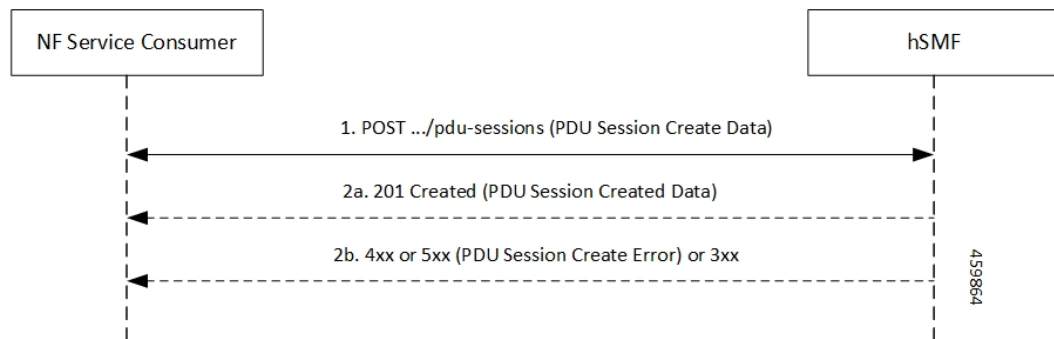
Figure 165: Create Service Operation on hSMF Call Flow
