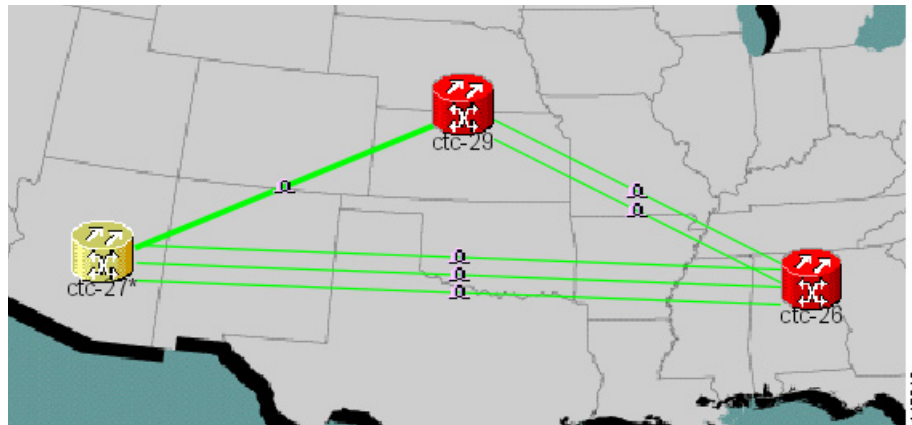
Figure 11-4 Network View with Local Link Consolidation
