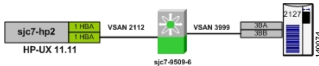
Figure 6-1 Single Switch IVR Topology
