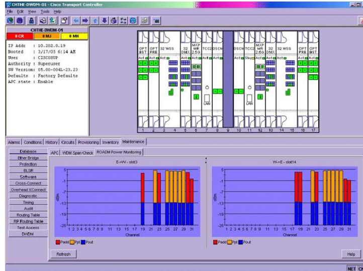
Figure 2 Cisco Transport Control Per-Channel Optical Power Monitoring
