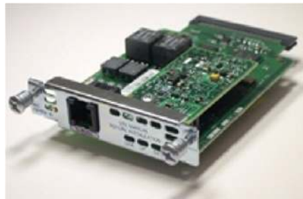
Figure 1. Cisco 1-Port G.SHDSL WAN Interface Card (part number WIC-1SHDSL-V3)
