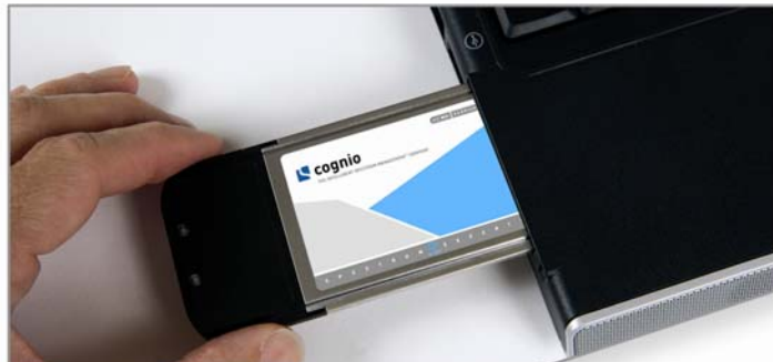
Figure 1 - Cisco's Spectrum Expert PC Card. An external antenna is also available. Source: Cisco Systems.
