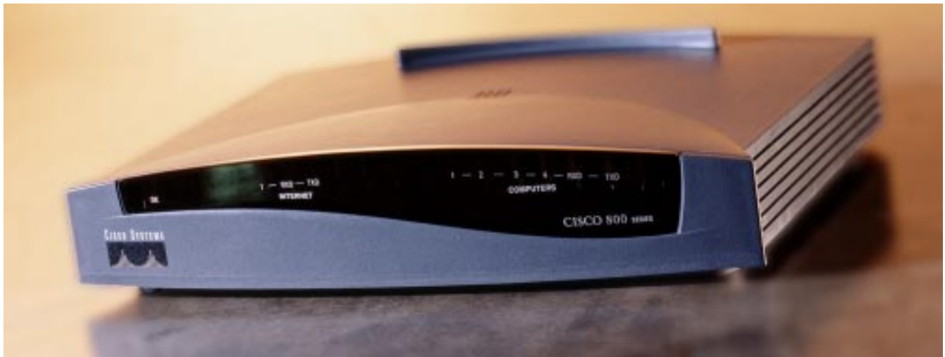
Figure 1 The Cisco 806 Broadband Gateway Router is a business-class, dual Ethernet router. It is ideal for a small business or enterprise telecommuter with Cisco IOS Firewall and VPN software to provide secure and reliable access to the Internet and corporate offices.
