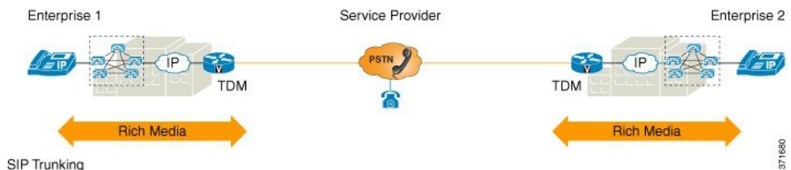
Figure 4: SIP Trunking Overcomes TDM Barriers
