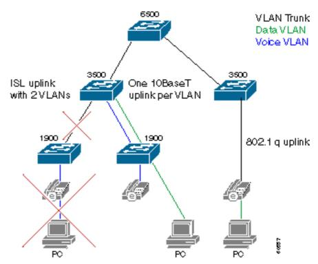
Phone and PC must be on separate ports on Catalyst 1900
