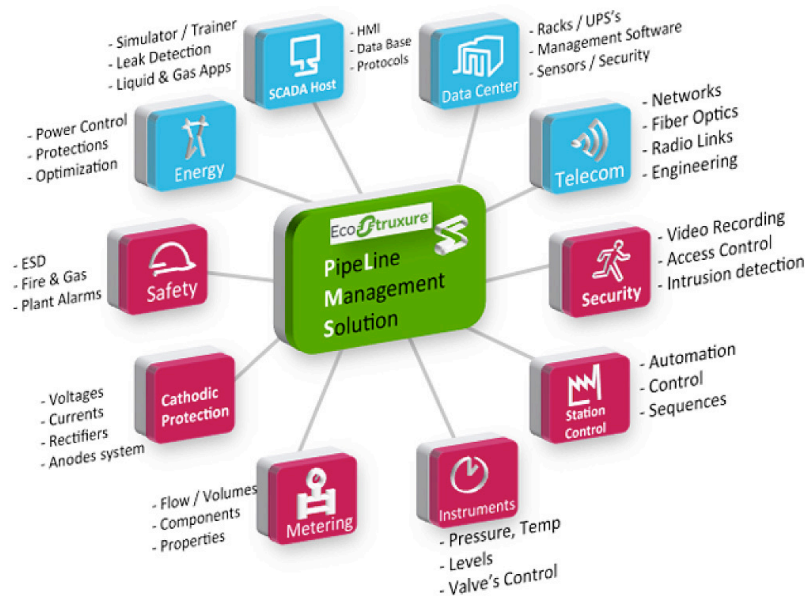
Figure 2. Pipeline Management System Modules
