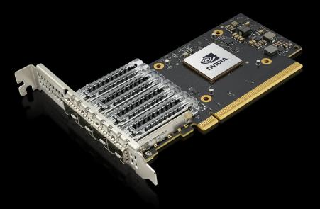
NVIDIA® ConnectX®-7 with four 25 gigabit Ethernet (GbE) ports is a remote direct-memory access (RDMA) over converged Ethernet (RoCE) network adapter that supports Ethernet protocol at 25 gigabits per second (Gb/s). It enables a wide range of advanced, scalable, and secure networking solutions for enterprise needs, from traditional workloads to the world's most-demanding AI, scientific computing, and hyperscale cloud data center workloads.
