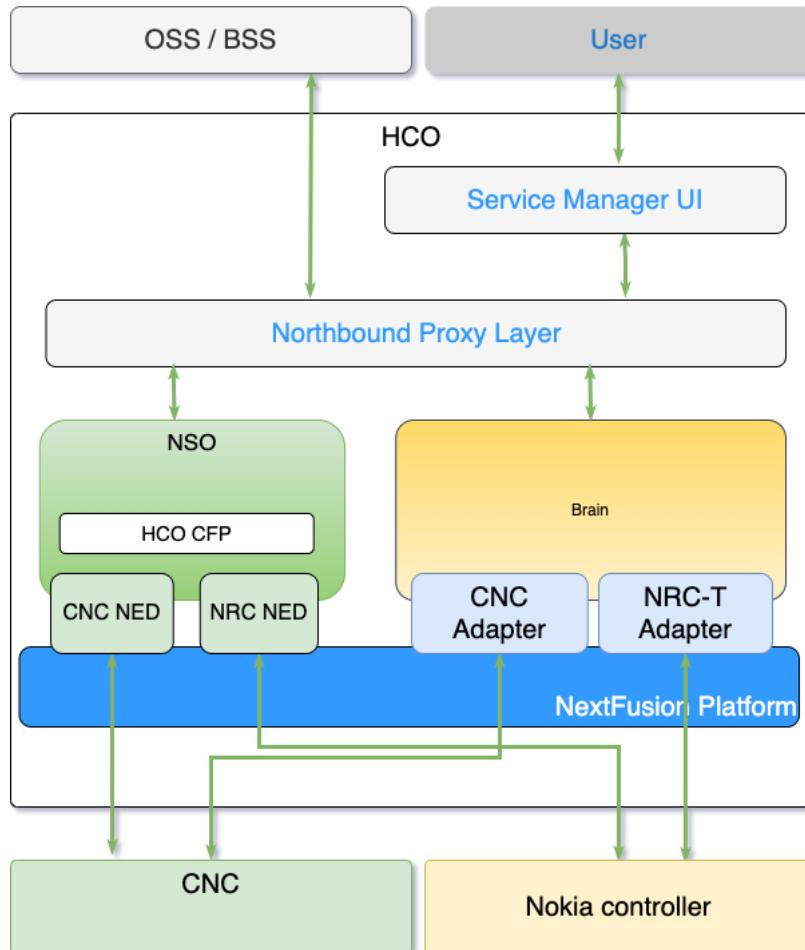
Service requests are submitted to NSO as service through the L2VPN and/or L3VPN data models. Each service deployment must specify a controller to which to push the service to. You can also define a global default controller. The FP interacts with the chosen controller NED in NSO to realize the services on the controller.
