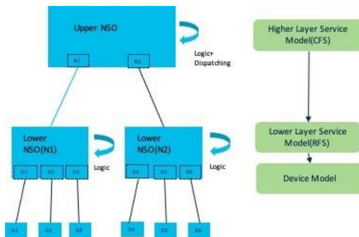
The upper-level node comprises the CFS packages for the T-SDN FP Bundle, the RFS NEDs, and other common packages and corresponding NEDs (such as core-fp-common and core-fp-common-ned).
