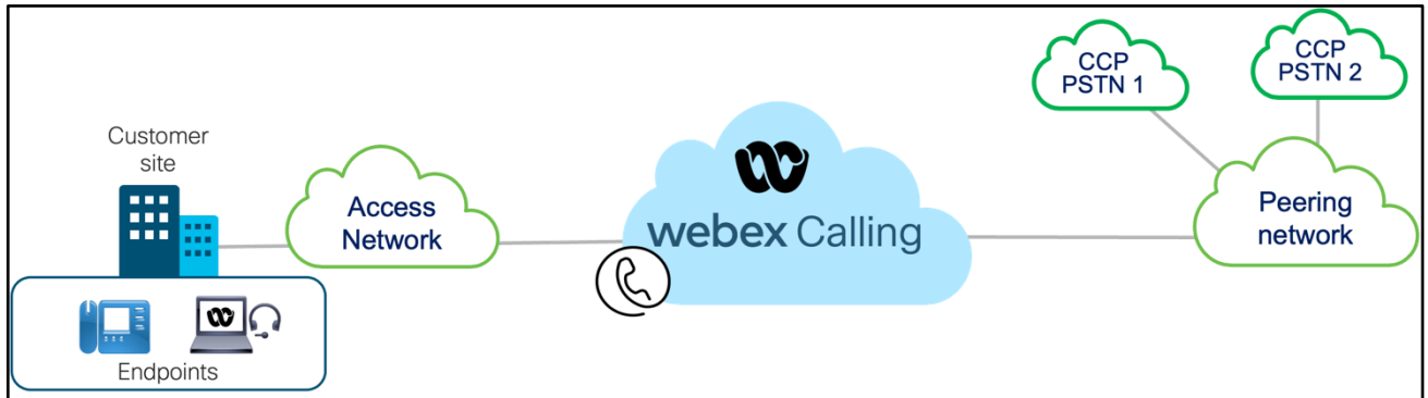
Figure 40 Cloud Connected PSTN
