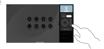
Use the controls to pan, tilt, and zoom the camera. Tap anywhere else on the screen to exit.
