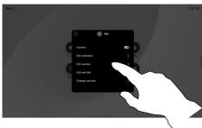
Edit the entry and tap Save on the keyboard to exit. Otherwise tap the back arrow on the contact card, or anywhere outside the card to exit.
