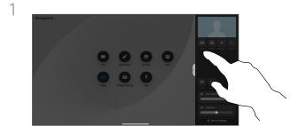
In or out of call, open the control panel and tap the **Camera** button. Or, tap the selfview image and then tap the Camera button there.
