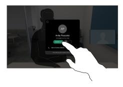
Tap the green Transfer **call** button. Talk to the person to confirm that transfer is OK. The person to be transferred is still on hold. 4
