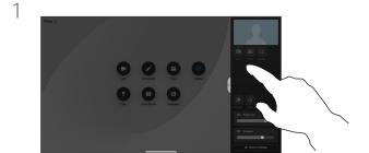
In or out of call, open the control panel and tap the **Camera** button. Select **Auto**
