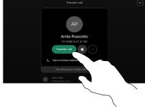
Tap the green **Transfer call** button. Talk to the person to confirm that transfer is OK. The person to be transferred is still on hold.
