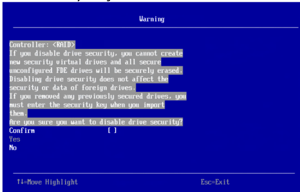
Figure 97 Disable Drive Security Warning
