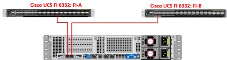
Figure 5 HX-Series and Cisco UCS C-Series Server Connectivity
