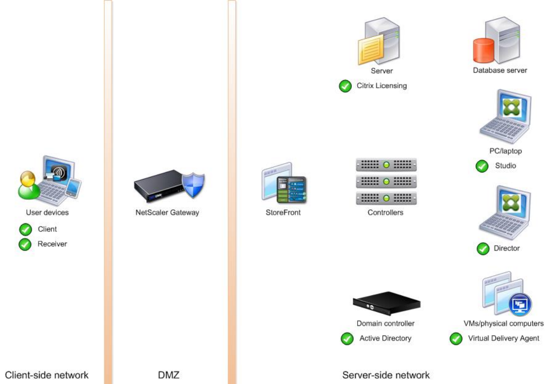
Figure 34 Example of a Distributed Components Configuration
