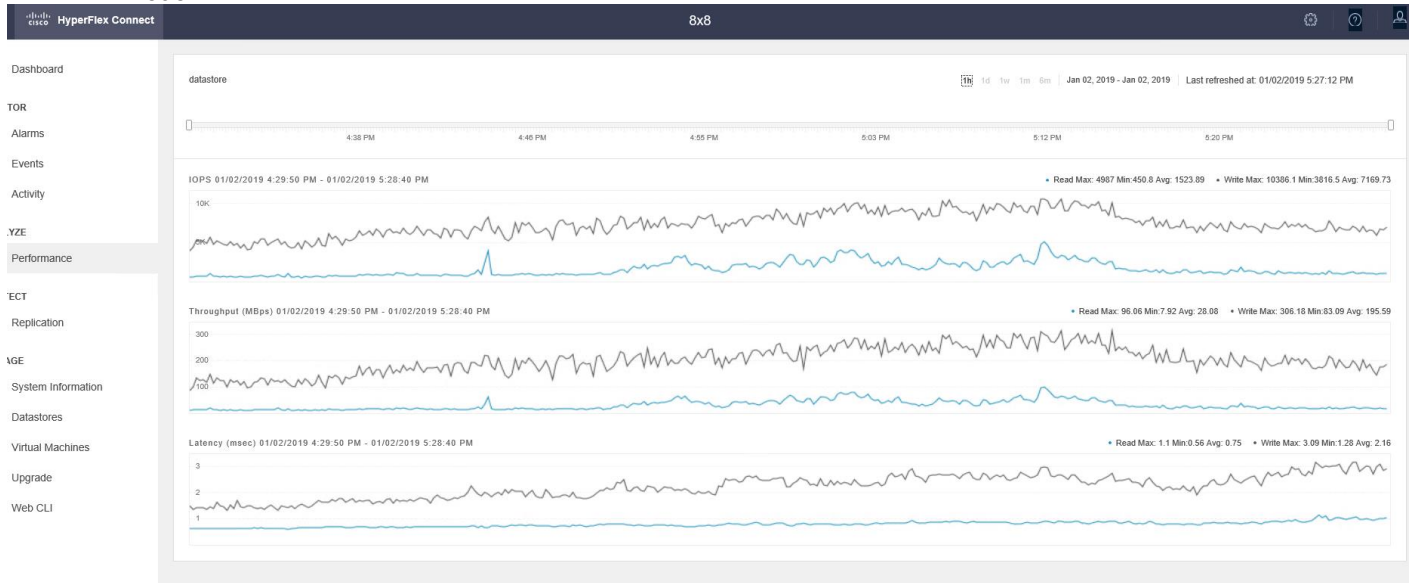
Figure 56 HyperFlex Cluster WebUI Performance Chart for Knowledge Worker Workload Running 2000 User Test on 16 Node
