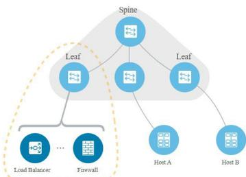
The diagram illustrates a network topology with a central Spine switch connected to three Leaf switches. The Leaf switches are further connected to Host A and Host B. A dashed orange circle highlights a service cluster consisting of a Load Balancer and a Firewall, which is connected to the Leaf switches.
