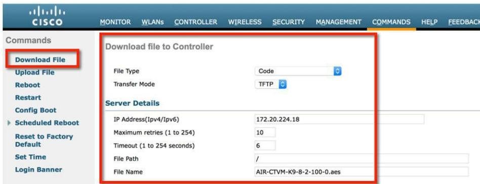
The screenshot shows the Cisco Web GUI interface for downloading a file to the controller. The left sidebar contains a 'Commands' menu with 'Download File' highlighted. The main content area is titled 'Download file to Controller' and contains the following fields:
