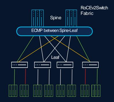
Traffic efficiency through pinning rules Map traffic from each downlink to the desired uplink
