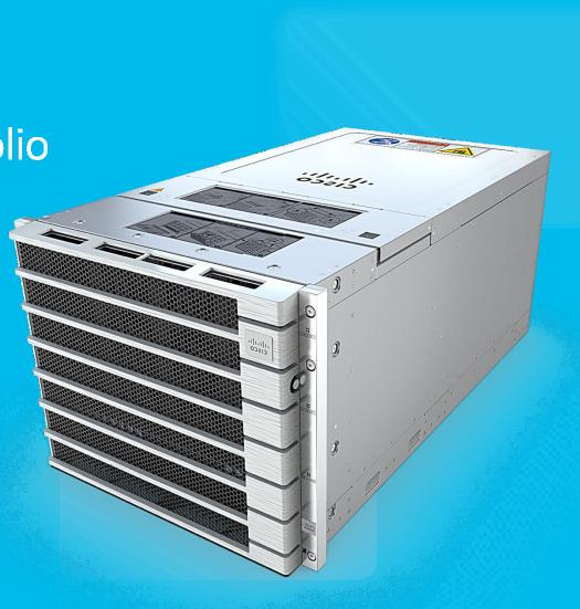
NvidiaHGXwith 8NvidiaH100,H200or AMD Mi300XGPUs 2AMD4th Gen EPY® Processors
