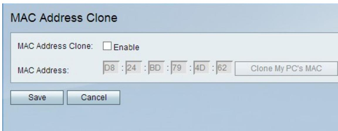
The screenshot shows the 'MAC Address Clone' configuration page. At the top, the title 'MAC Address Clone' is displayed. Below it, there is a checkbox labeled 'MAC Address Clone:' with the text 'Enable' next to it. Underneath, the 'MAC Address:' field is populated with the hexadecimal value 'D8 : 24 : BD : 79 : 4D : 62'. To the right of this field is a button labeled 'Clone My PC's MAC'. At the bottom of the page, there are two buttons: 'Save' and 'Cancel'.
