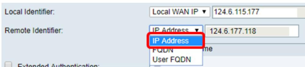
The screenshot shows the 'Remote Identifier' dropdown menu. The 'IP Address' option is selected and highlighted with a blue box. The dropdown menu is open, showing the following options: 'IP Address', 'FQDN', and 'User FQDN'. The 'IP Address' option is currently selected, and the value '124.6.177.118' is displayed in the adjacent text field. The 'Local Identifier' field above it shows '124.6.115.177'.
