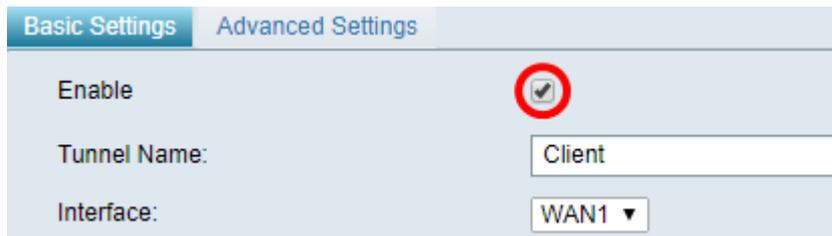
The screenshot shows the 'Basic Settings' tab for a VPN configuration. The 'Enable' checkbox is checked and circled in red. The 'Tunnel Name' field contains the text 'Client'. The 'Interface' dropdown menu is set to 'WAN1'.
