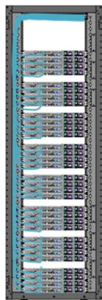
Figure 16. Standardized Breakout Layout Methodology with 32 servers
