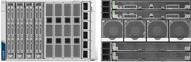
Figure 1. Cisco UCS X9508 Server Chassis, front (left) and back (right)
