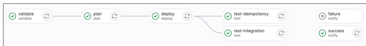
Figure 7. Network infrastructure CI/CD pipeline example
