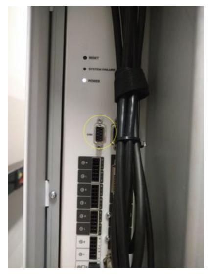
Step 2. Get the COM port number and set the baud rate to 115200 bps.
