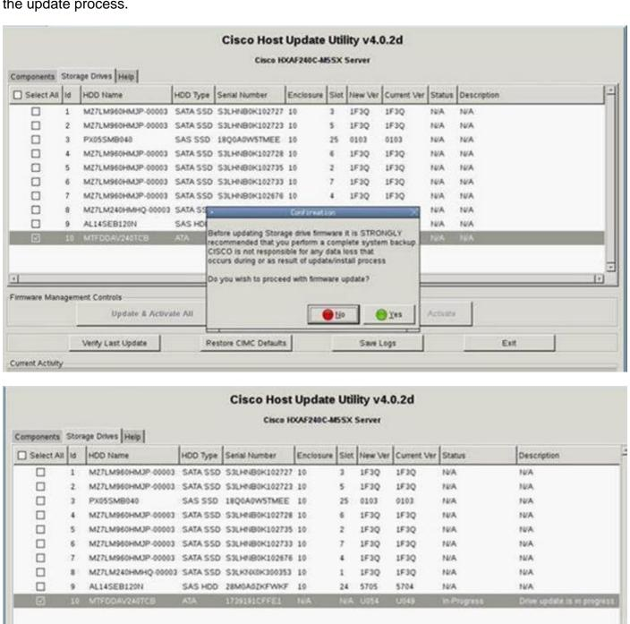
Step 9. Select M.2 drive and click **Activate.** Hit **Yes** in order to proceed with the activation process as shown in the image.
