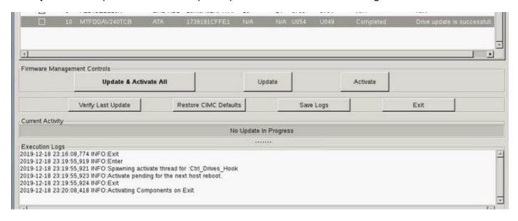
Step 10. Select **Exit** in order to activate the new firmware on the M.2 drive. The system should reload automatically. Un-map the HUU from the KVM session. The system should boot successfully to the operating system.
