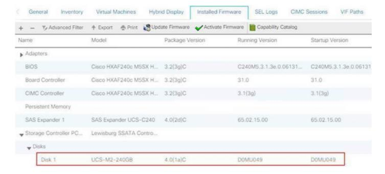
You need to upgrade the firmware on M.2 drive from D0MU049 to D0MU054 prior to upgrading the HX node to 4.0.4e C-bundle.
