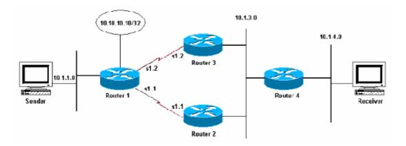
In the figure above, Routers 2 and 3 are talking HSRP on subnet 10.1.3.0, and Router 2 is the active router. Routers 1, 2, and 3 are talking Enhanced Interior Gateway Routing Protocol (EIGRP), and Router 4 has a static default route to the HSRP virtual address.
