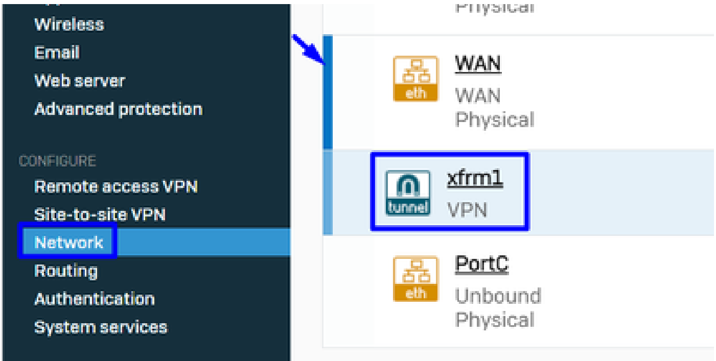
Sophos - Network - Tunnel Interface
