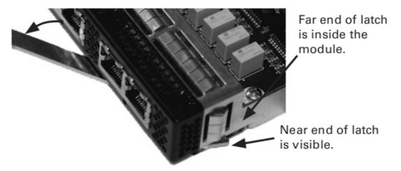
Step 3: Insert the module into the slot until the far end of the latch is inside the slot and the near end of the latch touches the outside of the slot.
