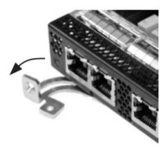
Step 3: Slide the module out of the slot.
