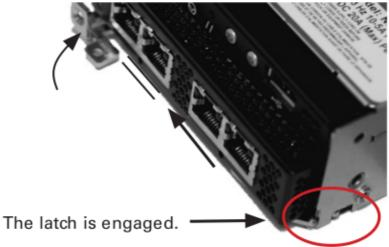
Do NOT use excessive force. If the latch does not engage, remove and realign the module, then try again.
