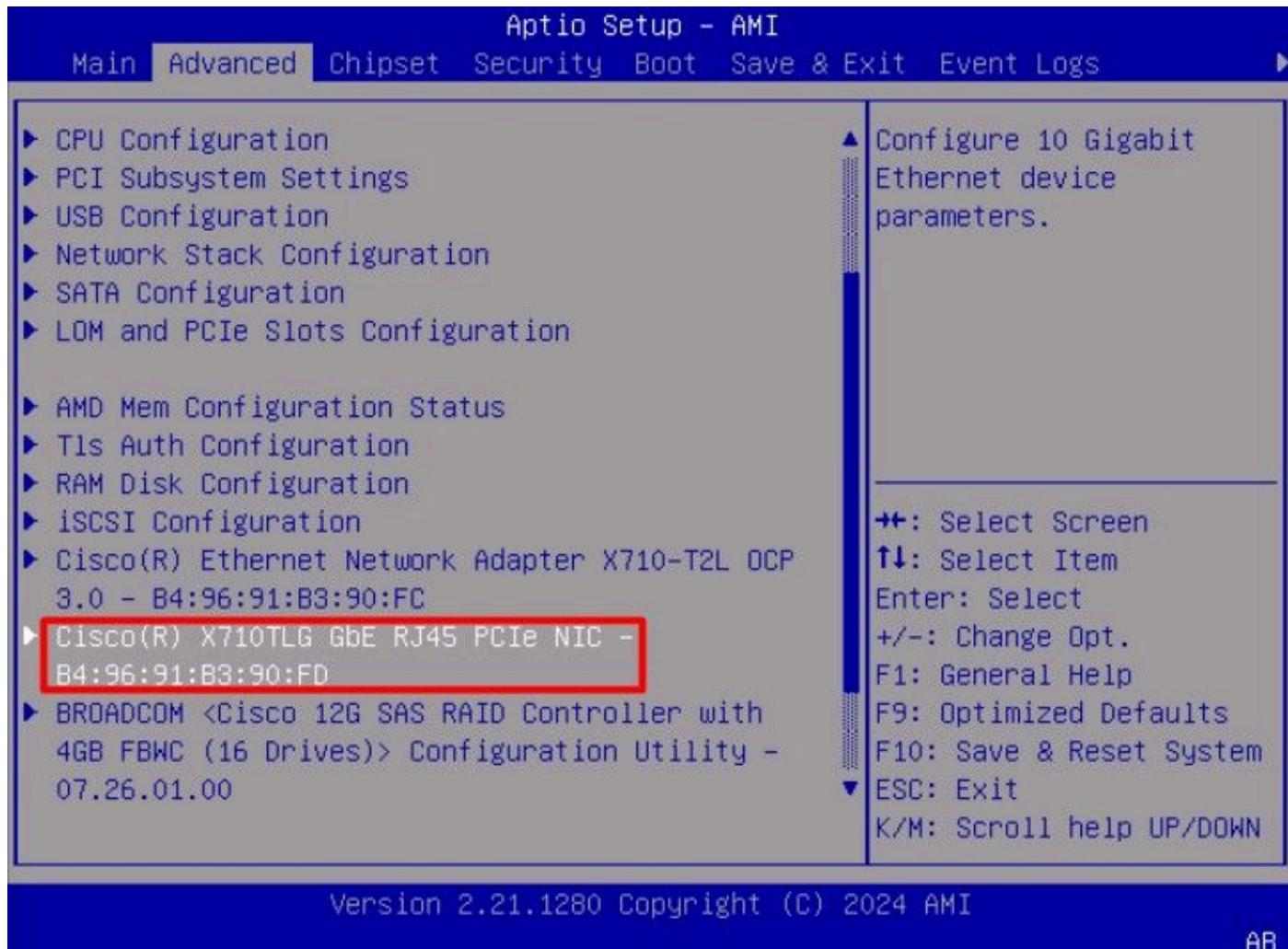
**Step 5.** Inside the network adapter option, validate the **Link Status** is **Connected**.
