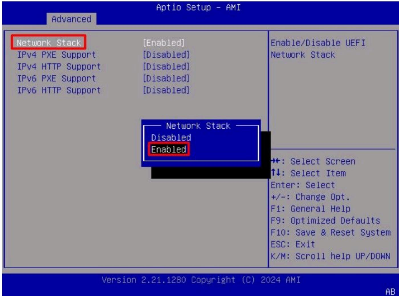
**Step 4.** Once the network stack is enabled, select the network adapter to use for iSCSI boot.
