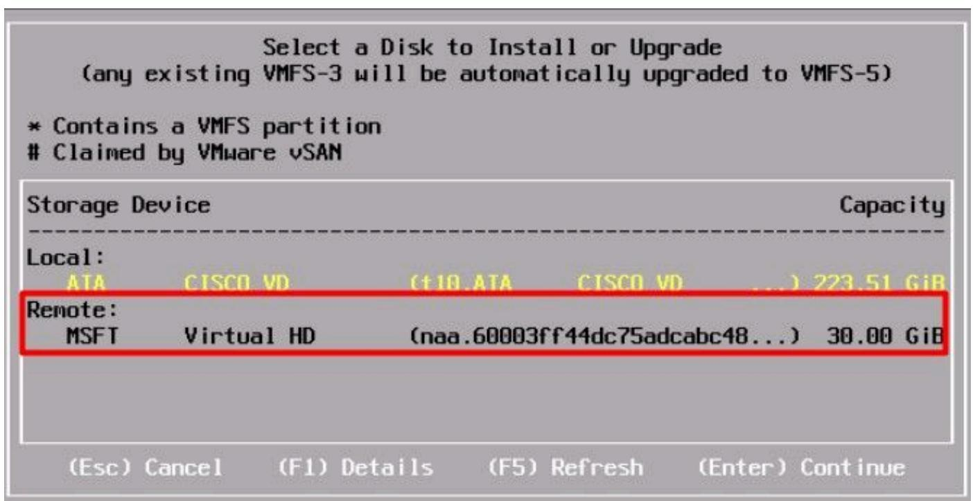
**Step 18.** Continue the installation process using the remote storage. Once it finishes, reboot the server and press F2 to enter the server BIOS settings. In the BIOS settings, select the **Boot Menu** and move the option **VMware® ESXi** to the **Boot Option # 1**:
