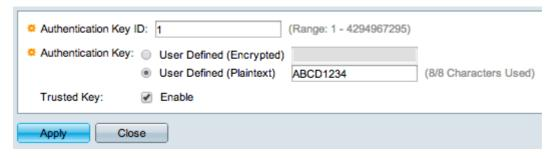
Step 5. Enter the number that is used to identify the SNTP Authentication key internally in the Authentication Key ID field.
