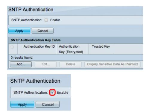
Step 2. Check the **Enable** check box in the SNTP Authentication field to require authentication of an SNTP session between the switch and an SNTP server.
