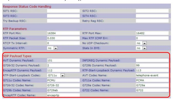
Step 3. Enter the number on which the sender and receiver must agree for the session event in the *AVT Dynamic Payload* field. The range is from 96 to 127. The default is 101.
