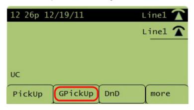
Step 1. Press the **GPickUp** softkey.
