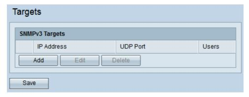
Step 2. Click **Add** to add a new SNMP target. A WAP device supports a maximum of eight targets.
