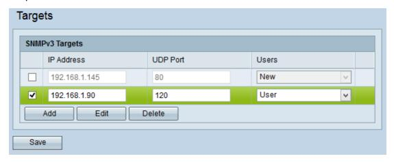
Step 9. (Optional) To edit an existing target, check the target check box in the SNMPv3 Targets table and click **Edit**. Make the desired changes and click **Save**.
