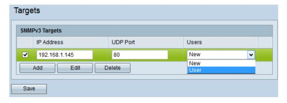
Step 3. Check the check box that corresponds to the new target added.
