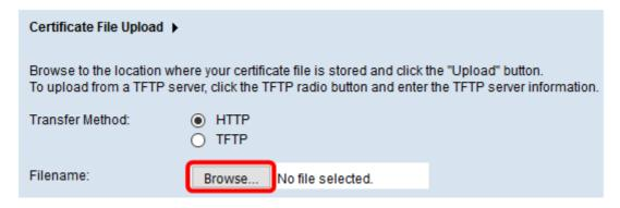
Step 3. (Optional) If you chose TFTP in Step 1, enter the name of the certificate file in the *Filename* field. The TFTP server is used to automatically transfer boot files within devices and is very simple.
