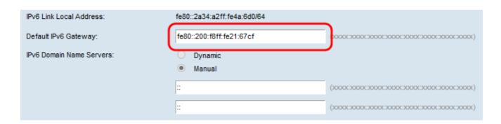
Step 8. If you selected **DHCPv6** in Step 2, choose the radio button from the *IPv6 Domain Name Servers* field for how you would like DNS servers to be allocated.
