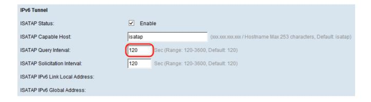
Step 4. In the *ISATAP Solicitation Interval* field, specify how often (in seconds) the WAP device should send router solicitation messages to ISATAP routers that the WAP discovers through the DNS query messages. The WAP device sends the router solicitation messages only when there is no active ISATAP router. The default value is 120 seconds.
