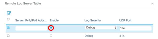
Step 5. In the *Server IPv4/IPv6 Address/Name* field, enter the address or the name of the remote syslog server. The format must either be in IPv4, IPv6, or a Fully Qualified Domain Name (FQDN).
