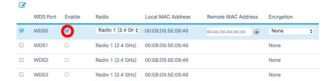
Step 7. From the Radio drop-down list, choose the radio interface to apply the WDS settings.
