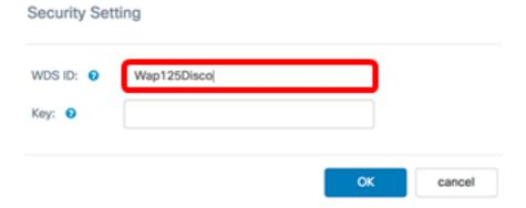
Step 12. Enter the authentication key for the WAP in the *Key* field. This information should be the same in all the WAP devices that connect to a WDS. The required key length should be eight to 63 characters.
