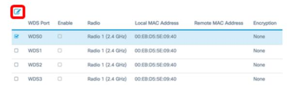
Step 6. Check the **Enable** check box to enable the WDS port.
