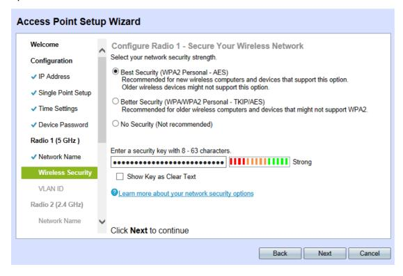
Step 27. Click the corresponding radio button for the desired network security method. The methods are as follows:
