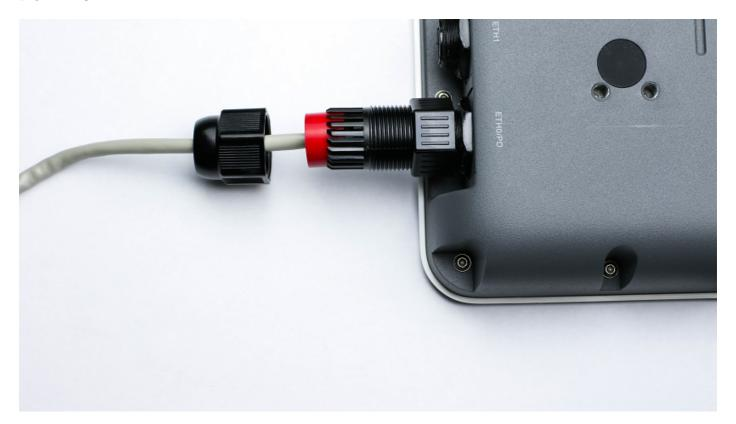
Step 6. Insert the thick rubber gasket into Part B of the weather-proof connector.
