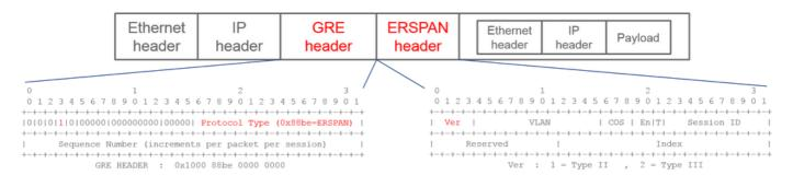
If the sequence field is activated by the S bit, this must be ERSPAN type II or III. The version field on the ERSPAN header identifies the ERSPAN type. In ACI, type III is not supported as of 03/20/2016.
