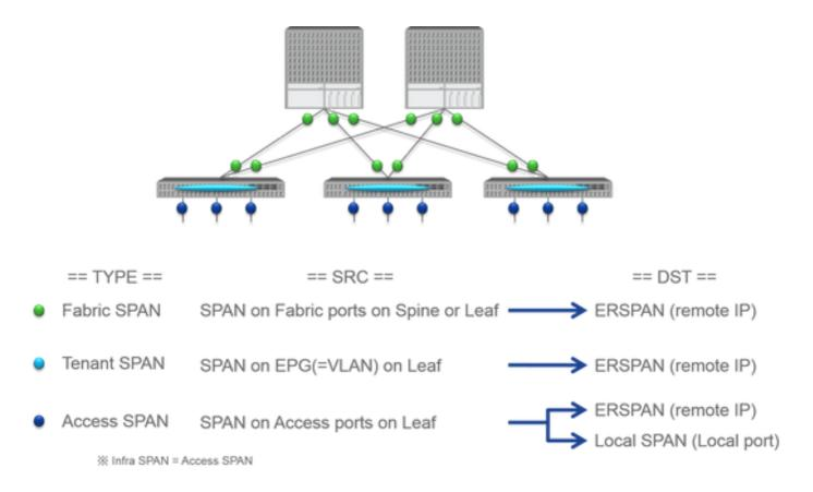
Cisco ACI has three types of SPAN; Fabric SPAN, Tenant SPAN and Access SPAN. The difference between each SPANs is the source of copy packets.
