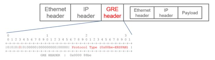
Type I does not use the sequence field on the GRE header. It does not even use the ERSPAN header which must follow the GRE header if it was ERSPAN type II and III. Broadcom Trident 2 only supports this ERSPAN type I.
